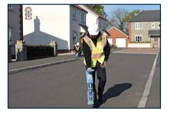
A locator for all industries 8 active and 4 sonde frequencies, 3 passive modes, power filters and other advanced features to provide efficient accuracy for locating and tracing burried utilities.
