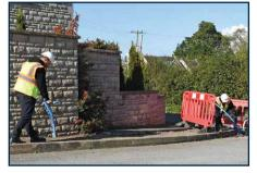
**Sonde mode** Locate non-conductive pipes or cable ducts and conduits at depths of up to 50' (15m).
