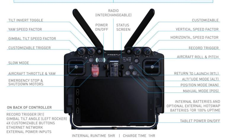
Use our CAD and API to integrate the Pilot Pro controller with your robotics system.
