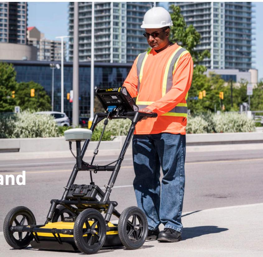
LMX200™ GPR complements traditional pipe and cable locators and allows you to locate and map targets below the surface.
