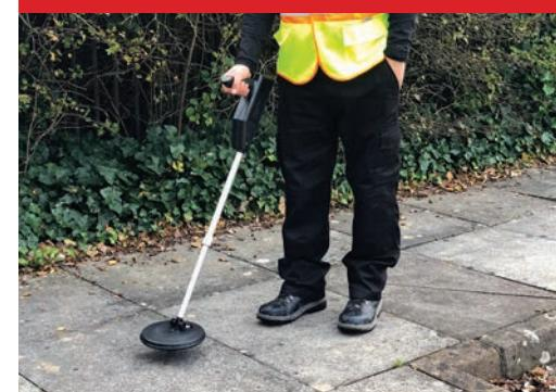
The RD312 locator sets a new standard of simplicity and reliability for finding valve box covers, vault covers, fuel tanks, reinforced rods in concrete and manhole covers, buried under road surfaces, gravel, grass or snow.
