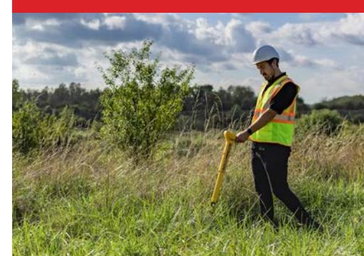
The GA-92XTd Locator detects the magnetic field of ferromagnetic objects. It responds to the difference in the magnetic field between two sensors that are spaced approximately 9.5 inches apart.
