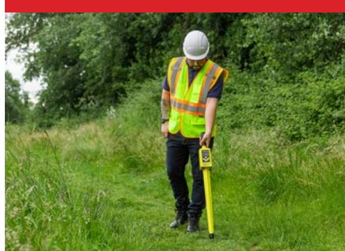
The GA-72Cd detects the magnetic field of iron and steel objects. It provides audio detection signals that peak in frequency when the locator's tip is held directly over the target.
