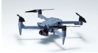
Small Aerial Photography Drone 1.7kg/65cm wide/IP43
