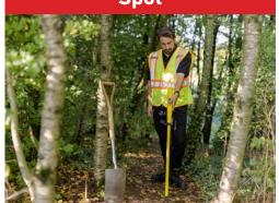
The Schonstedt Spot Magnetic Locators detect the magnetic field of iron and steel objects.
