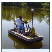
Map depth to bedrock and geological stratigraphy Locate underground storage tanks (UST) Detect sinkholes Conduct bathymetry and sub-bottom profiling
