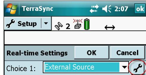
If using Integrated SBAS, no additional settings are needed as the SBAS correction is referenced to WGS 84. However, if a VRS, single base station or Beacon correction source is specified, you must know the datum of the correction source and enter it here.
