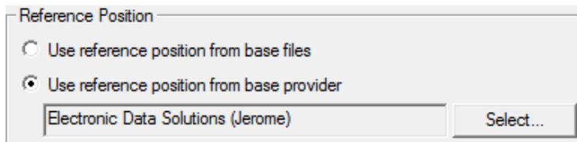
The default choice is to use the reference position contained in Trimble's base station list, which has been compiled from details submitted by base station operators and is presented in terms of ITRF00. This is the option selected, in the Pathfinder Office Differential Correction Wizard (v3.1 and newer).
