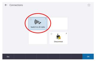
The radio settings are sent to the SX12 using the existing Wi-Fi connection and then applied when the controller connects to the instrument. The instrument will then change to LRR mode.
