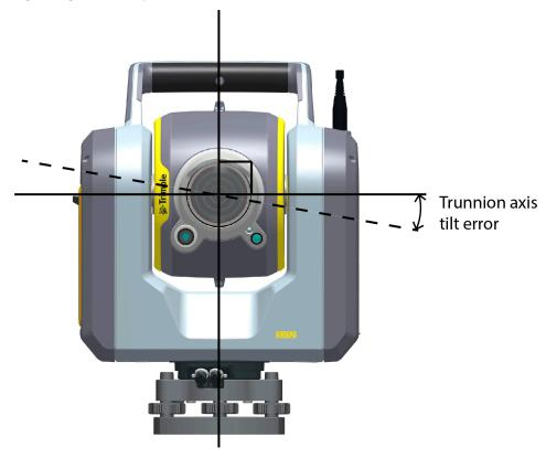
The trunnion axis tilt error is measured at the factory and stored in the instrument as a correction value. This correction value is then applied to correct the horizontal angle value and the telescope is automatically repointed using Surepoint technology.
