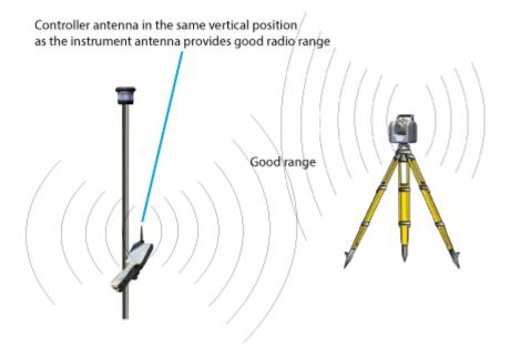
Good radio range with controller antenna in the same vertical position as the instrument antenna
