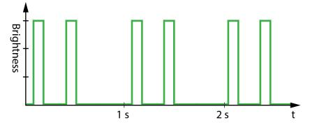
Laser pointer flashing pattern to indicate that the laser pointer is not aligned with the crosshair
