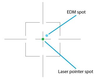
In STD mode the crosshair is aligned to the laser pointer. The EDM spot position relative to the crosshair and laser pointer will change slightly depending on instrument temperature, instrument face, and range. For a cold instrument in face 1, the EDM spot is up and to the right from the laser pointer, as shown above. For a warm instrument in face 1, the EDM spot is down and to the left relative to the laser pointer. In face 2, the opposite is true.
