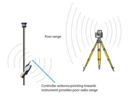
Poor radio range with controller antenna not in the same vertical position as the instrument antenna
