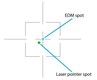
In TRK mode the crosshair is aligned to the EDM. The EDM spot position relative to the crosshair and laser pointer will change slightly depending on instrument temperature, instrument face, and range. For a cold instrument and in face 1, the EDM spot is up and to the right from the laser pointer, as shown above. For a warm instrument and in face 1, the EDM spot is down and to the left relative to the laser pointer. In face 2, the opposite is true.
