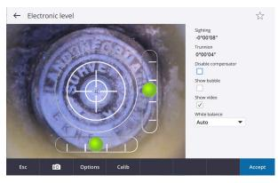
**NOTE** – The orientation of the plummet camera is aligned to a user standing at the back side of the instrument. See Set up over a point, page 16.
