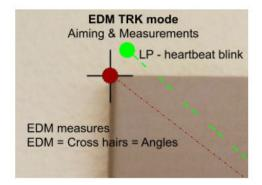
To avoid the unintentional high accuracy use of a laser pointer with tracking mode, the laser pointer has a unique "heartbeat flash pattern" when the EDM is in tracking mode. This flash pattern is consistent across all modes of the laser pointer (standard, low-light, extended range flashing), though the intensity will vary between the modes.
