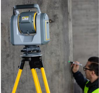
The laser pointer's small size, color, and power all contribute to its exceptional visibility. The small laser spot is achieved using focusing lenses. The color is green, which is more visible to the average human eye than red. The power, though always Laser Class 1, can be set to three different modes to suit the environment and maximize visibility.
